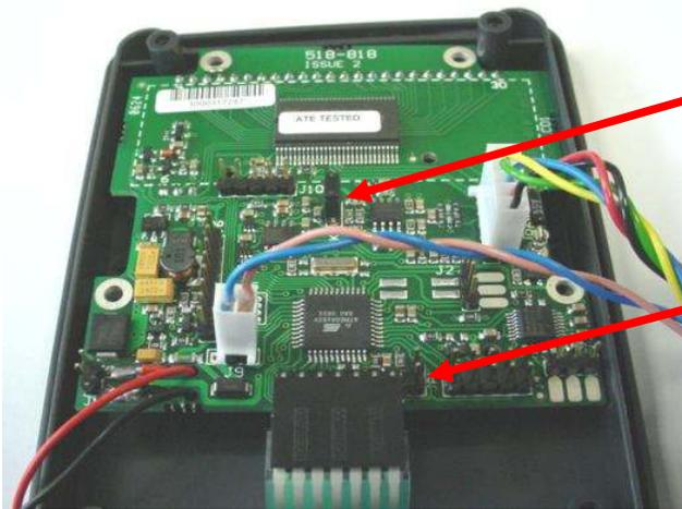
Sensitivity link should be in this position for use with sensors, with sensitivities <math>\lt; +/- 5\text{mV/V}</math>
