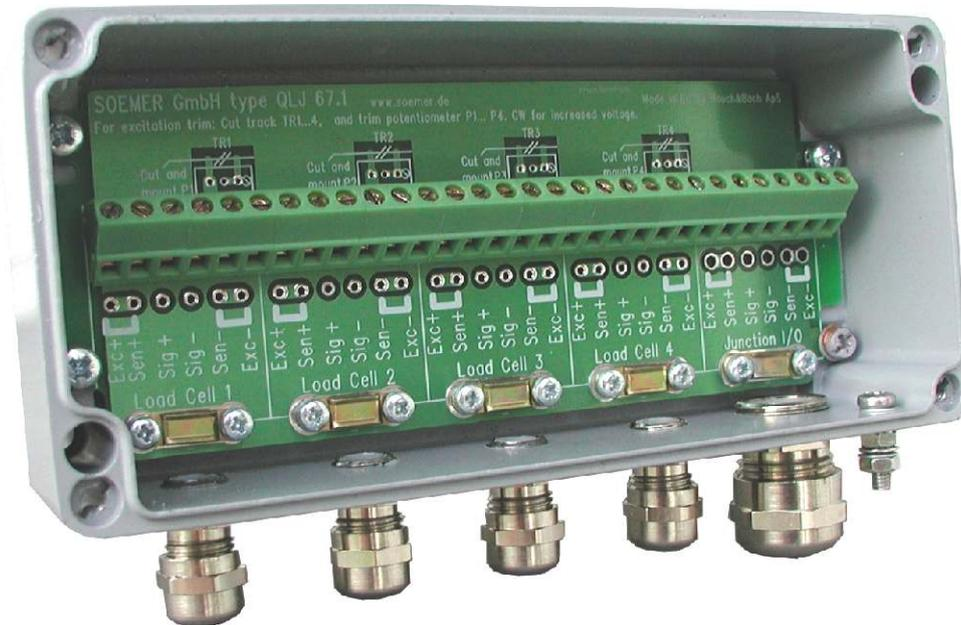
This junction box is designed to connect up to 4 load cells (in parallel) to the instrumentation/load cell amplifier. More than 4 load cells can be connected (if the instrumentation can drive more than 4 load cells) by cascading 2 or more QLJ 67.1 together.
